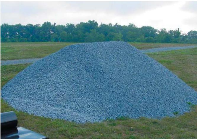
Fig. 1.9 Gravel used under traditional porous asphalt system.
