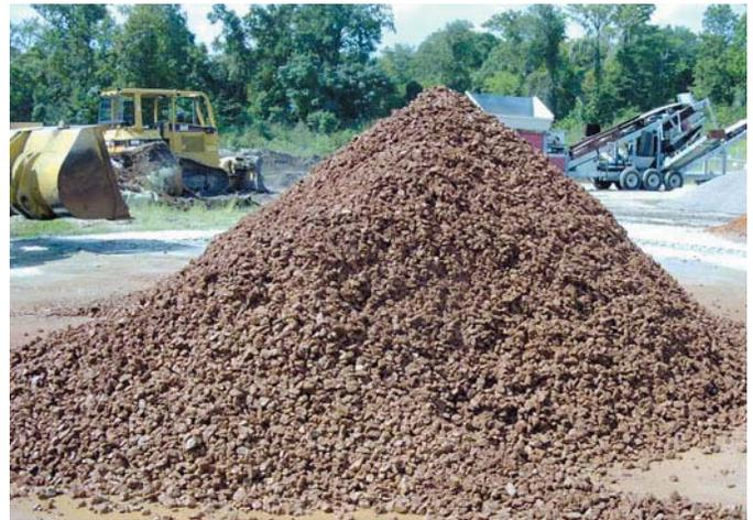
Fig.1.10 CU-Structural Soil® Matrix. Soil particles within the media adhere to gravel.
