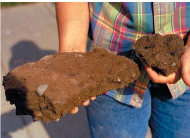
Fig. 1.18 Compacted soil from a typical construction site. Lack of structure prohibits root penetration and growth.
